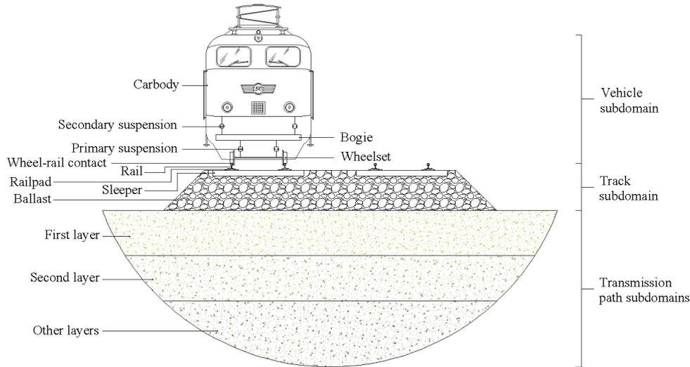
Figure 2: Longitudinal section view of the vehicle/track/soil subdomains.
