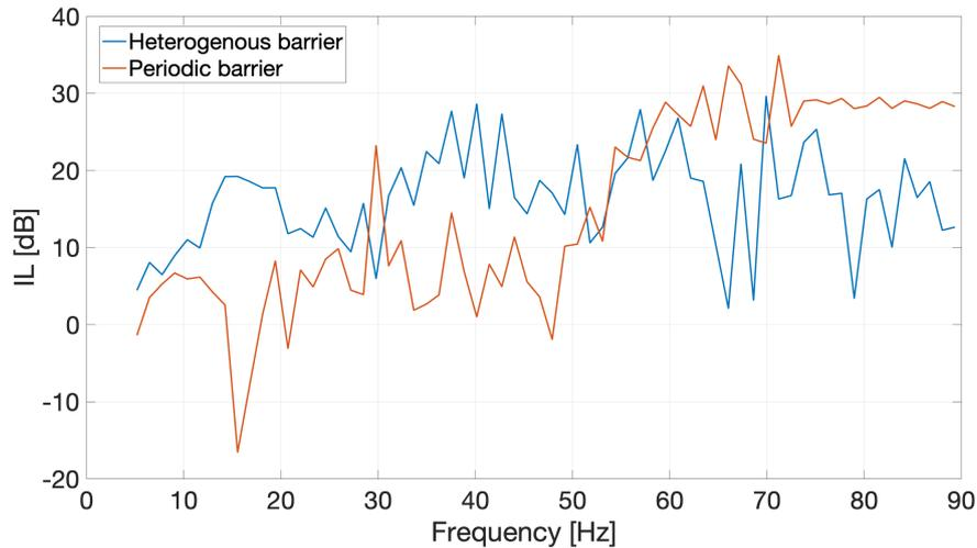
Figure 10: Comparison of insertion losses for the heterogeneous and the periodic barrier
