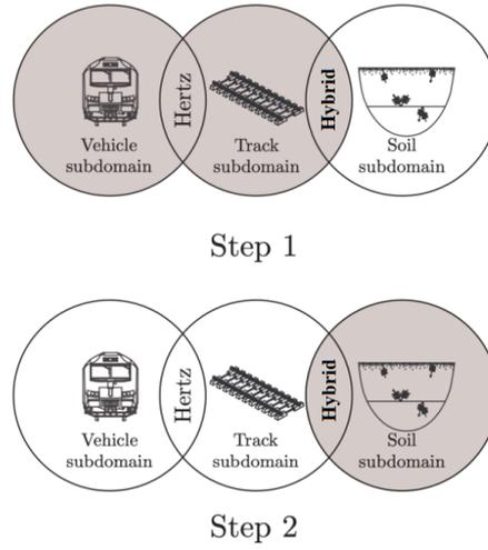
Figure 3: Vehicle/track/soil model, decoupled between the ballast and the soil [14].
