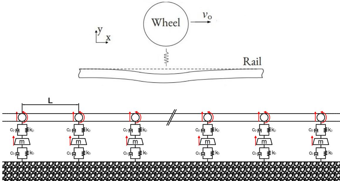
Figure 4: Mono-wheel vehicle at a speed  $v_0$  and track/foundation coupling
