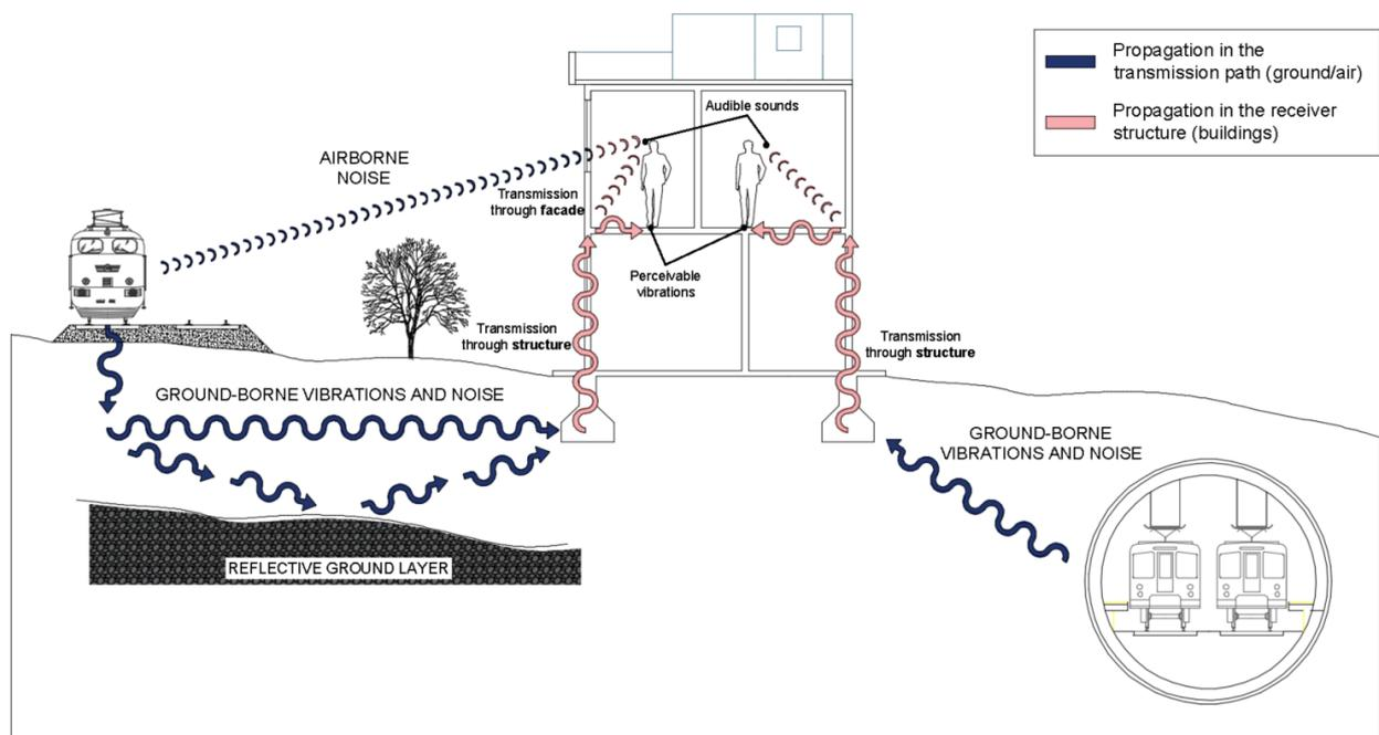
Figure 1: Surface and underground railway mechanism effects and transmission paths of air-borne noise and ground-borne vibrations and noise [2].
