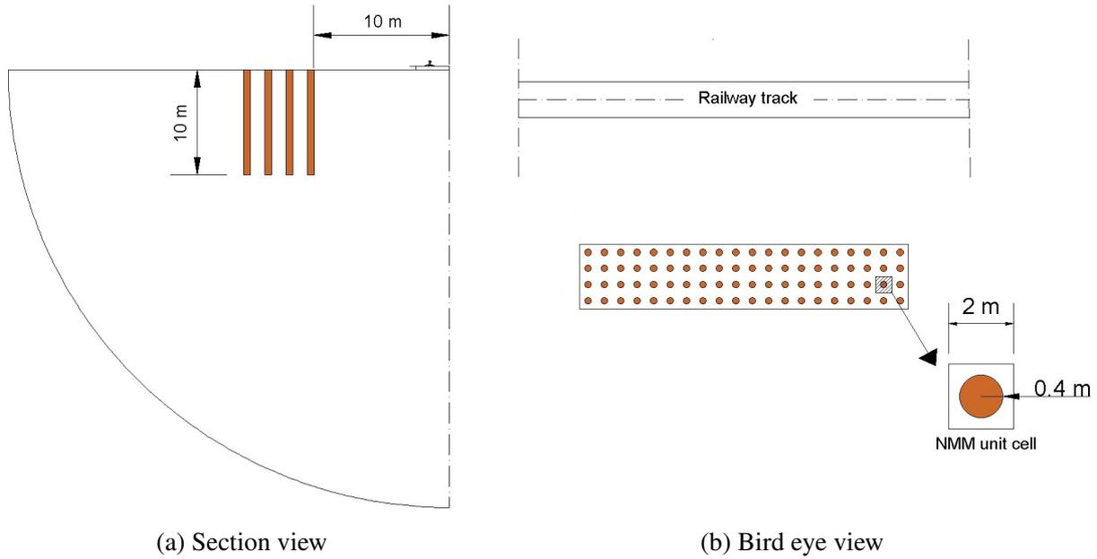
Figure 6: Distribution of the trees array in the model, with details of the natural metamaterial units.
