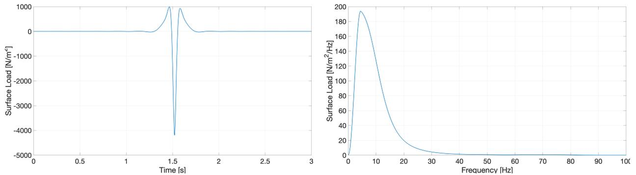
Figure 5: Time history (left) and spectrum (right), of an example of load applied at one sleeper position.
