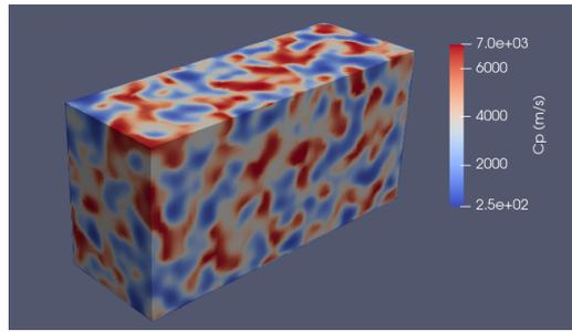
Figure 8: Random realization of the pressure wave velocity  $C_P$  of the barrier
